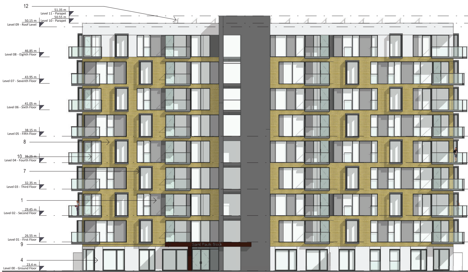
FIG. 47 - NINE STOREY BLOCK FRONT ELEVATION
